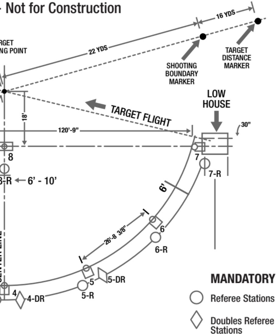
markers plus or minus six inches; target emergence elevation, high house, plus or minus three inches from level of Station 1, low house plus or minus three inches from level of Station 7. Station levels within plus or minus nine inches of Station 8 level. Mandatory referee positions should be marked.
